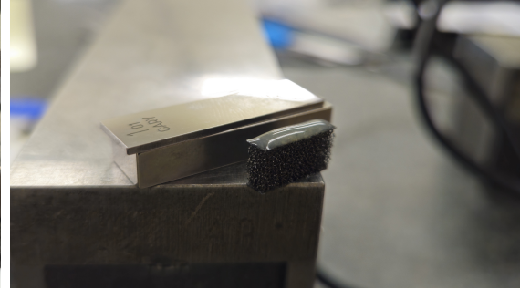
(b) Adding glue on the cured foam + fleece.
