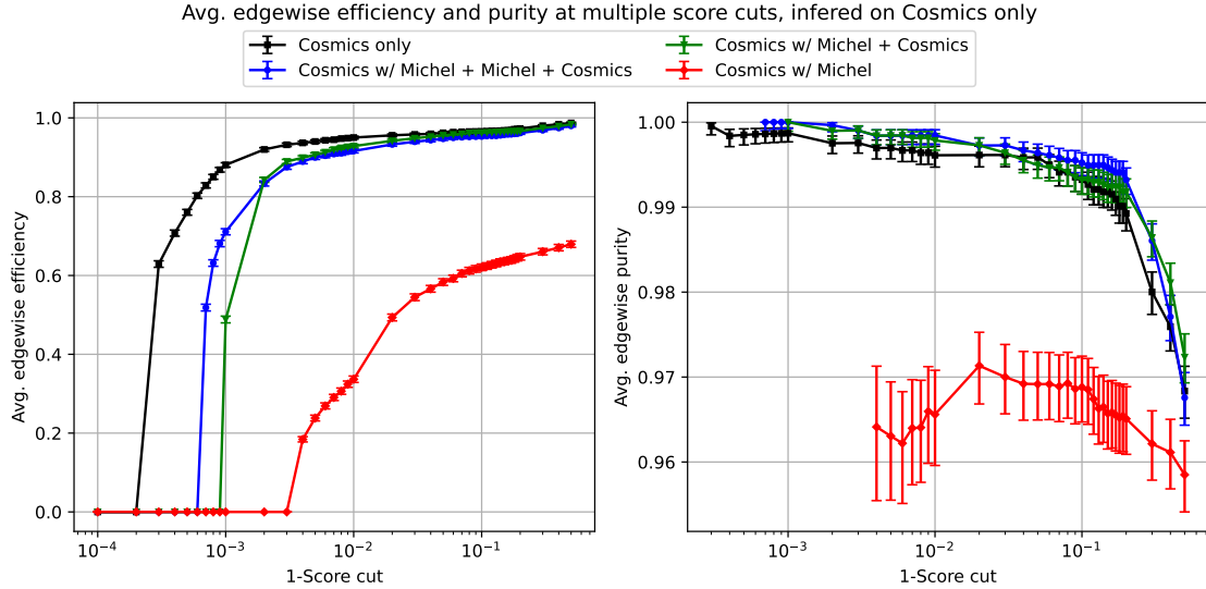
Figure 3.4: Average edgewise efficiency (left) and average edgewise purity (right) of different GNNs inferred on 1000 test set frames of the cosmics-only data sample as functions of 1—the score cut threshold. The different colors correspond to the different training sets of the inferred GNNs. Errors are calculated as the 1\sigma Clopper-Pearson confidence interval.
