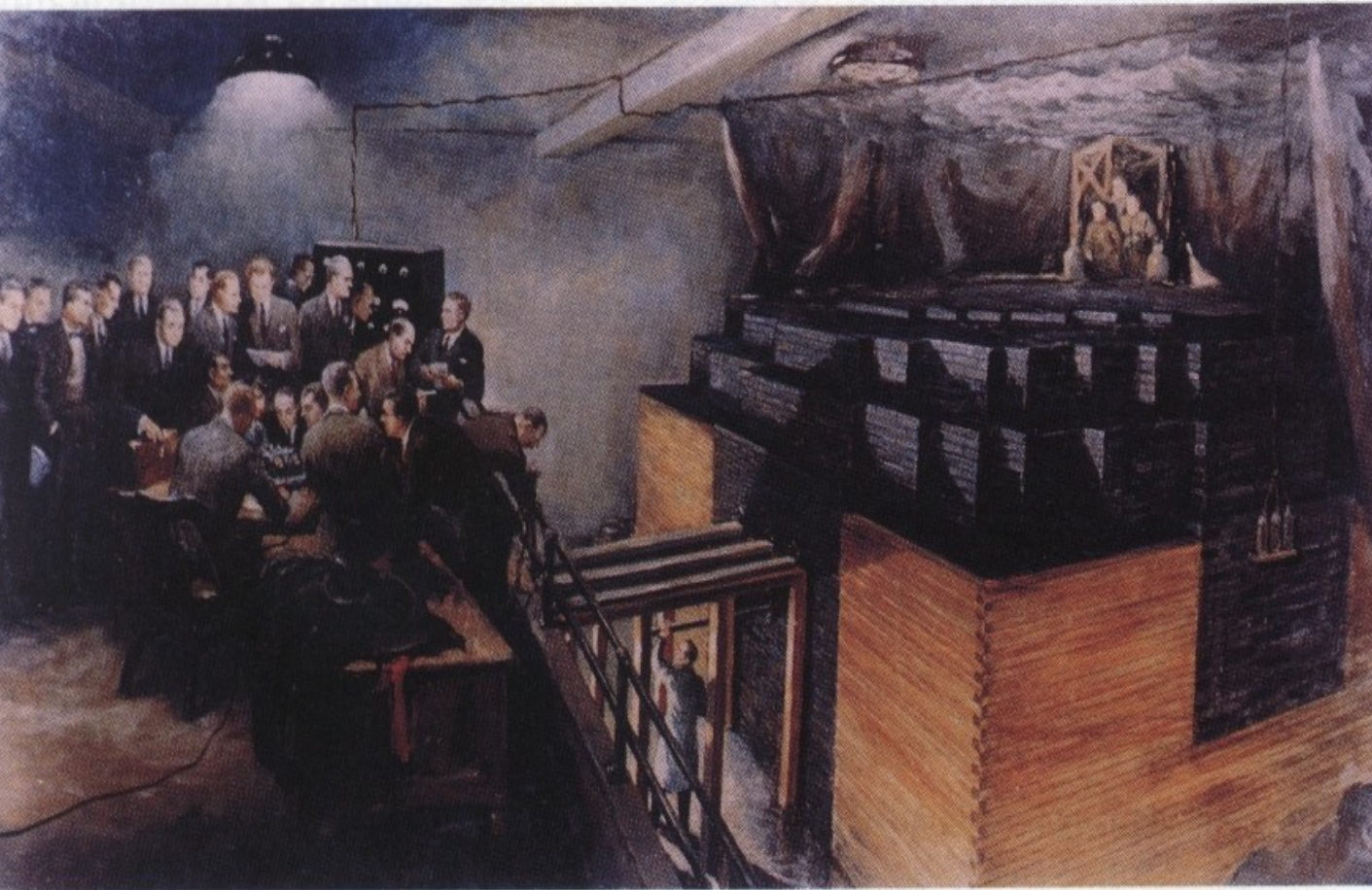
FIGURE 31-4 Color painting of the first nuclear reactor, built by Fermi under the grandstand of Stagg Field at the University of Chicago. (There are no photographs of the original reactor because of military secrecy.) Natural uranium was used with graphite as moderator. On December 2, 1942, Fermi slowly withdrew the cadmium control rods and the reactor went critical. This first self-sustaining chain reaction was announced to Washington, by telephone, by Arthur Compton who witnessed the event and reported: “The Italian navigator has just landed in the new world.”
