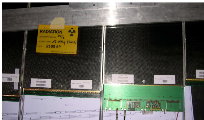
Figure 10: Photograph of the preamplifier board connected to a module.
