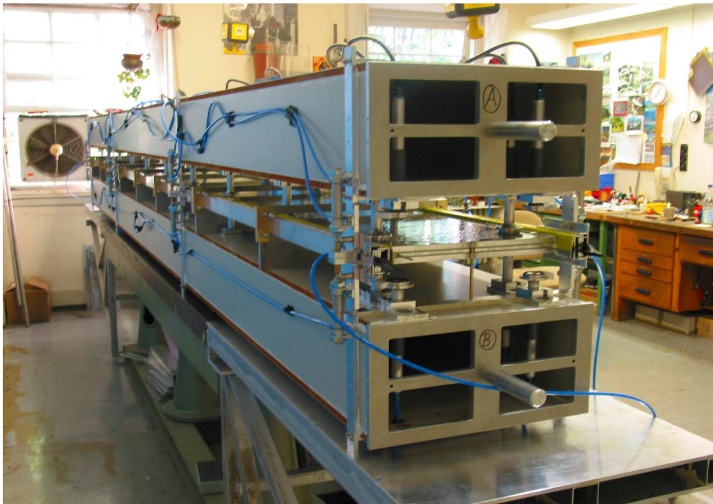
Figure 6: Gluing of the test box.
