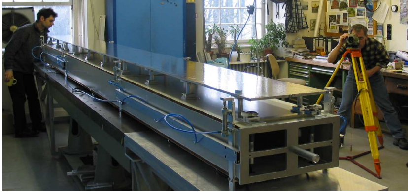
Figure 3: Top: Sketch of panel handling tool with sandwich panel underneath. Bottom: Panel fixed on panel handling tool, during measurement of panel straightness with a theodolite.
