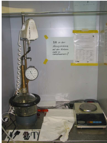
Figure 1: Mixing station for the preparation of the adhesive.
