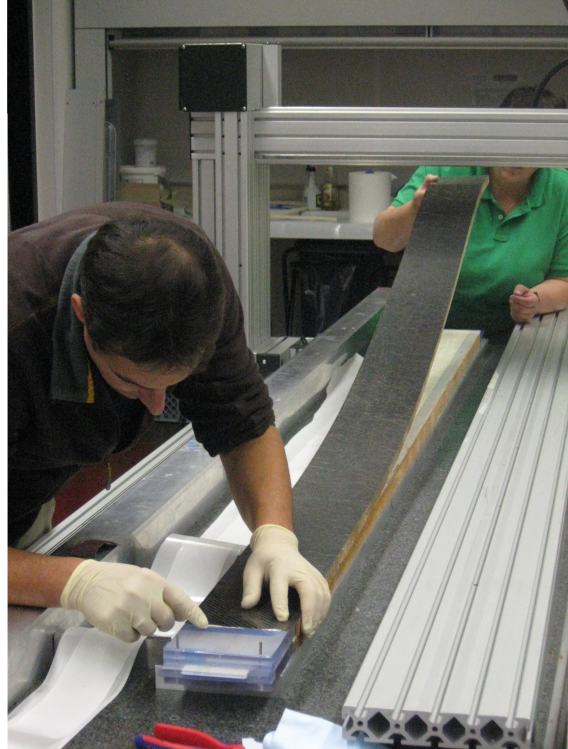
Figure 7: Gluing a half panel to a sub-module while constructing a testbeam module made of one sub-module. In the final production this step is performed for eight sub-modules at a time.
