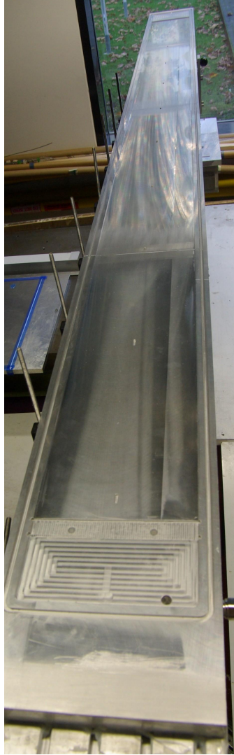
Figure 1: 2.5m casting mold used to cover the raw fibre mats with a thin, protective layer of glue.
