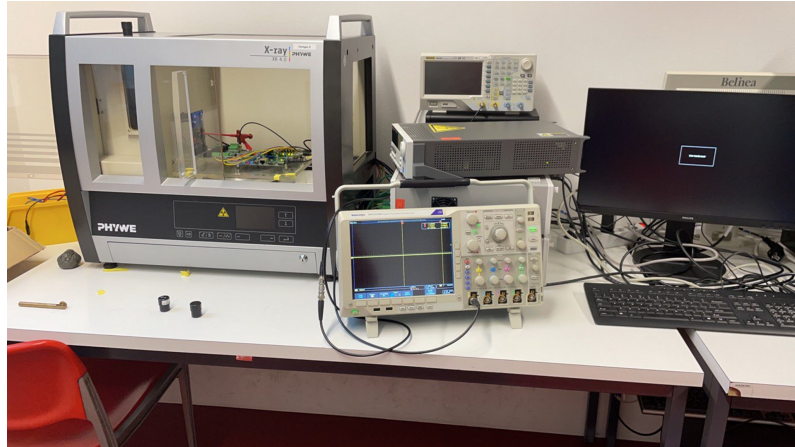
Fig. 6.5 X-ray setup at Heidelberg University. This setup was used for all X-ray measurements presented in this thesis.
