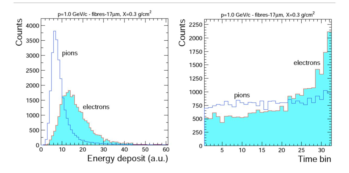
Figure 14.21: Integrated energy deposit for pions and electrons for a momentum of 1.0 GeV/c. A radiator with 17  $\mu$ m fibre has been used.
