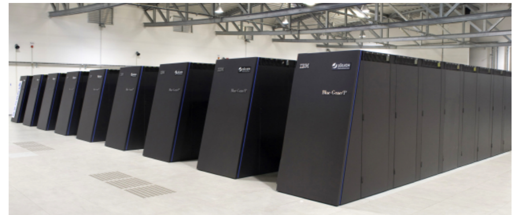
Example of a machine for lattice QCD: JUGENE in Jülich (294,912 processor cores, \sim 1 PetaFLOPS)
