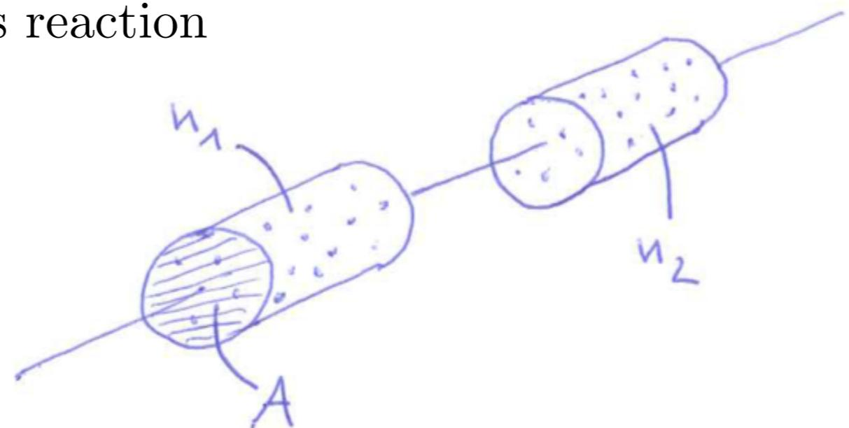
$n_1, n_2$  = numbers of particles per bunch in the two beams
